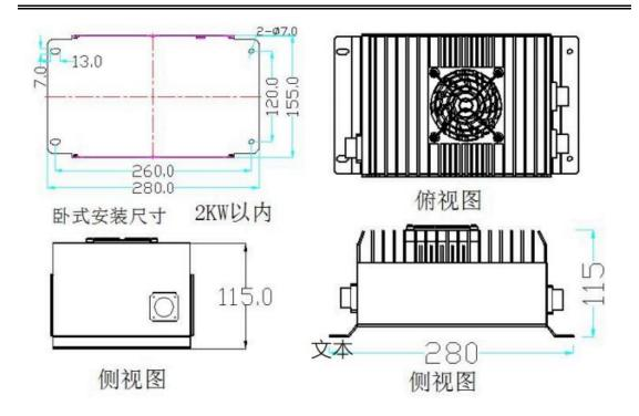
Horizontal mounting size within Q1-2KW
