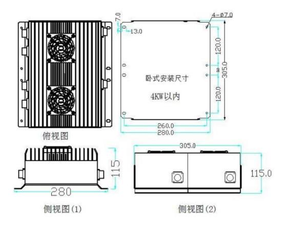
Horizontal mounting size within Q1-4KW
