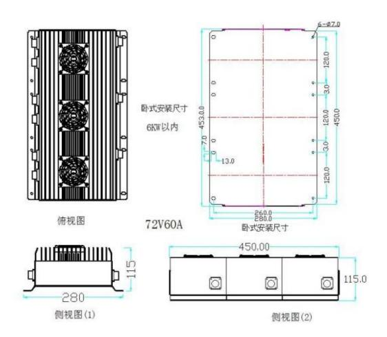
Horizontal mounting size within Q1-6KW
