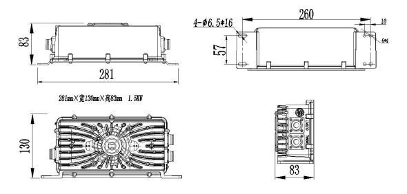
Horizontal mounting size within Q1-1.5KW
